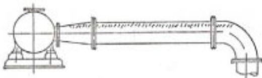
Showing how an air pocket may be formed when the suction pipe is bigger than the pump branch
