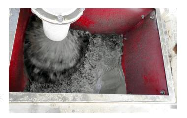
Our hydrocyclones are lined with special Polyurethane coating that has a high shore hardness of 93A, where most of the conventional hydrocyclones offer upto 70D.
